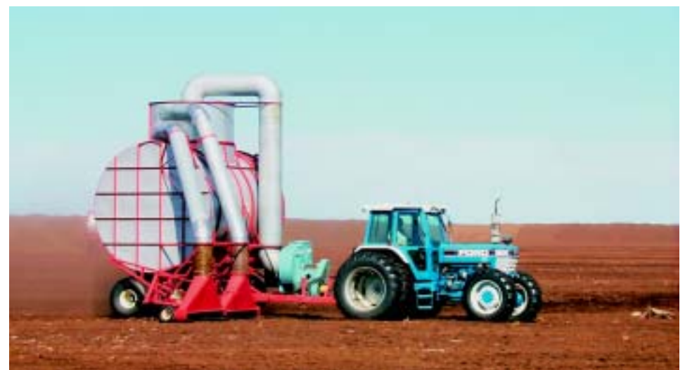
A tractor is pulling a harvester that vacuums up a small amount of peat moss, that has been exposed to the sun and air to dry, and holds it in the large bin. When the bin is full, the peat is dumped and later transported to a plant where it is screened, mixed, and packaged.
